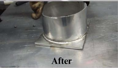
Post Weld Cleaning that will leave your welds free of contamination & discoloration
